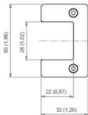
Figure 2.17 – Dimension and assembly of the three linear magnet models.
